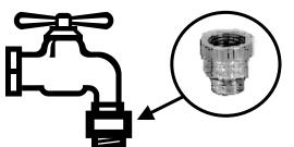
Another method of preventing backflow with a garden hose is using a device known as a vacuum breaker. Vacuum breakers are inexpensive devices that can be screwed onto your outside faucet. These devices will prevent contaminants from being siphoned back into your plumbing and the public water system.
