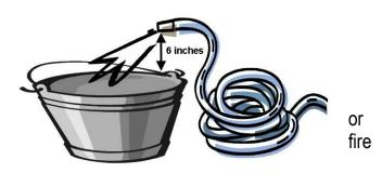
submerged in a source of contamination, the contaminant could be pulled back into the public water supply. This occurrence, known as backflow, can be prevented.
